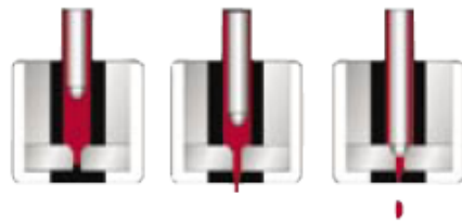
Figure 2. The ball-tip end of this technology pushes fluid through a narrow hole at the jet nozzle.
