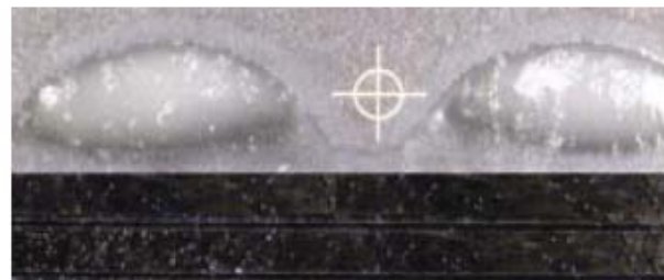
Figure 7. Normal underfill processes do not allow the accuracy needed to dispense around the fiducials without creating a void.
