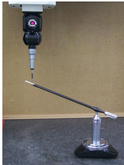
Figure 9. The Machine Checking Gage from Renishaw is a popular CMM interim test artifact.
