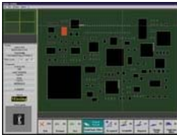
Figure 3. Repair station defect-location detail screen. Along the bottom, action buttons permit the recording and logging of all actions for future reference.
